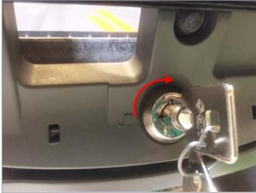
2. Unlock the dock by inserting the dock key into the dock lock and turning it counterclockwise until the lock is in the unlocked position.
