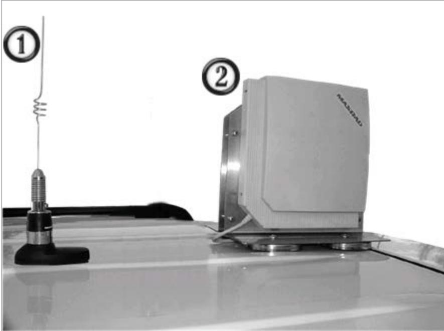
2. Route the antenna cables into the vehicle, taking care not to pinch or damage them.
