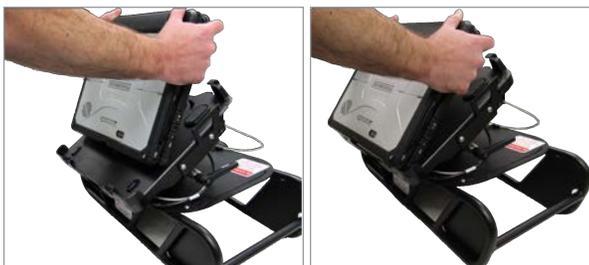
3. Slowly lower the back of the laptop onto the dock, ensuring that the laptop connectors and the dock connectors are aligned. The back of the laptop and the two dock latch hooks should look like this:
