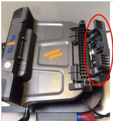
2. Holding the tablet in landscape position, angle the bottom of the tablet towards the dock's connectors.
