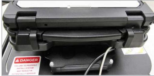
5. When the latch hooks are engaged the latch button on the front of the dock will move into the latched position.
