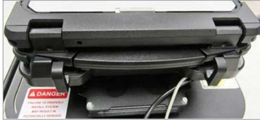
4. Gently push the back of the laptop down onto the dock until the latch hooks snap into place over the rear of the laptop.
