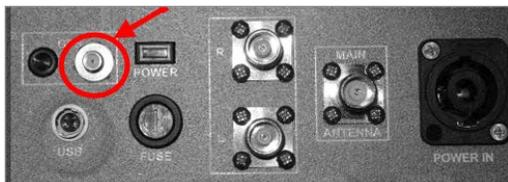
**Note:** When powered on, the LED indicator is lit to indicate that the GPS antenna is functioning properly. If the LED indicator is not lit, disconnect and reattach the cable to the GPS antenna connector. If the LED indicator is lit, continue installing your Mobile Collection system. If the LED indicator remains unlit, contact Itron support.
