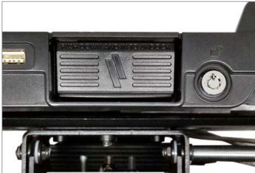
2. Holding the laptop at the top, angle the front edge of the laptop into the dock toward the latch button.
