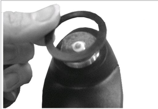
2. Press the antenna onto the thread nut of the antenna mounting base.
